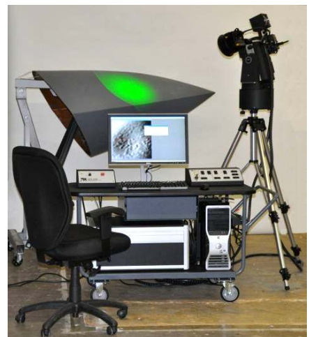
LTI-5100HD inspection of aircraft radome for damage and disbonds with optional TES-200 Thermal Stress Unit.
