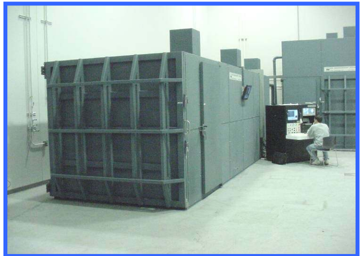
8' x 8' x 32' & 12' x 12' x 12' Vacuum Shearography Chambers
