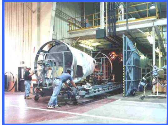
Fuselage Section being loaded into the LTI-9000 Production Shearography System
