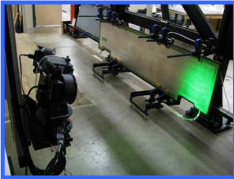
Shearography Camera & Exciter mounted on the X/Y 12' high x 20' long Shearography Gantry
