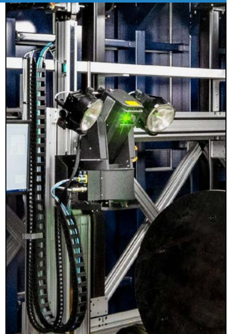
Above, a 5100 is mounted on a scan gantry in a vacuum test chamber.
